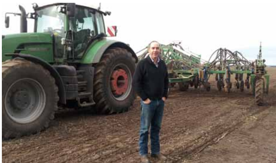
John Sheehan takes a break from direct drilling of oats into a lucerne paddock. The tractor has auto-steer, full GIS/GPS capability and is pulling a variable rate seeder.
