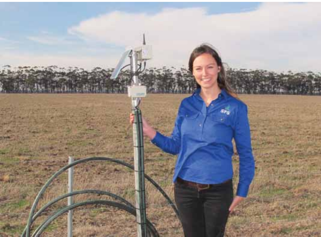
Elaina vanderMark with one of the 60 soil moisture probes being installed across southern Australia.
